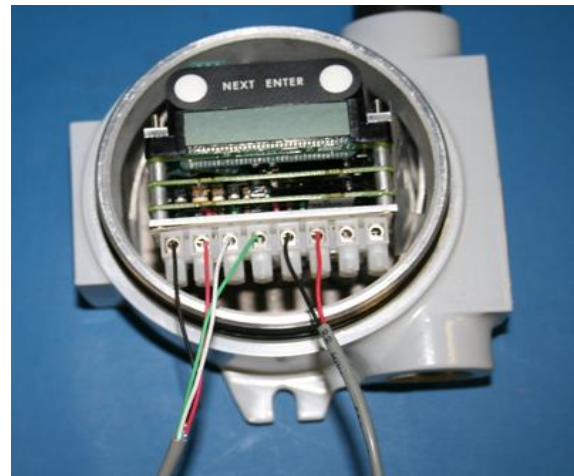
Figure 7: base radio with screw terminal
