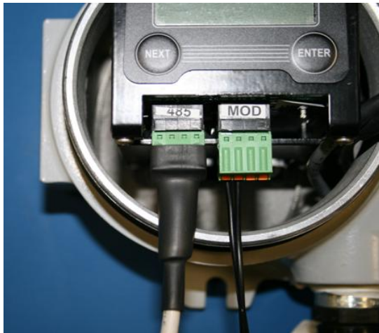
Figure 6: Base radio with spring loaded plugs
